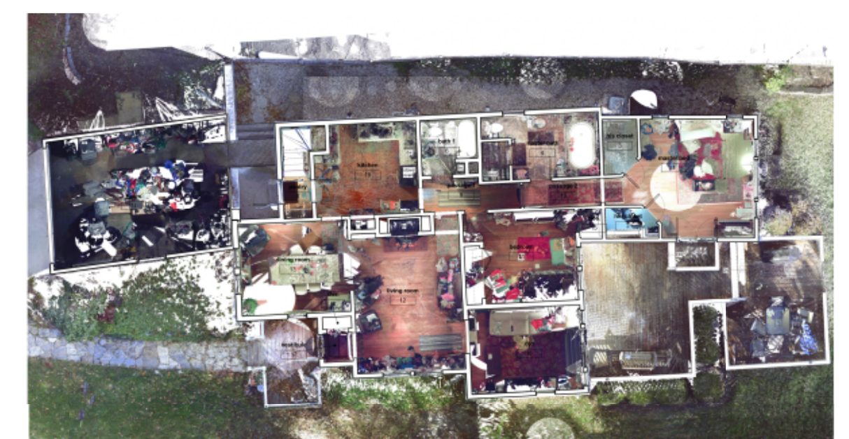
floor plan view of a residence - point cloud and linework
